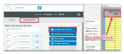
**Breakers:** either add in the quantity and catalog number or choose the **configure branch device button**. Update your **branch circuit quantity** and see your number of **Used Circuits**
